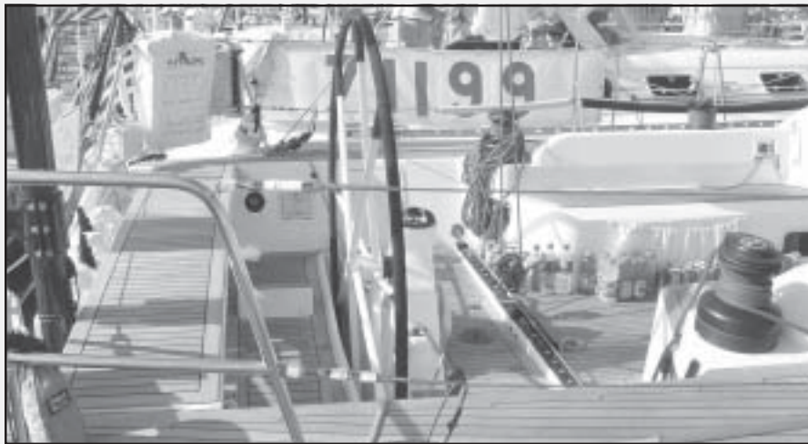
When a mainsheet traveler is this close to the helm, the pedestal and any guards must be designed to avoid snagging the sheet during a jibe.
