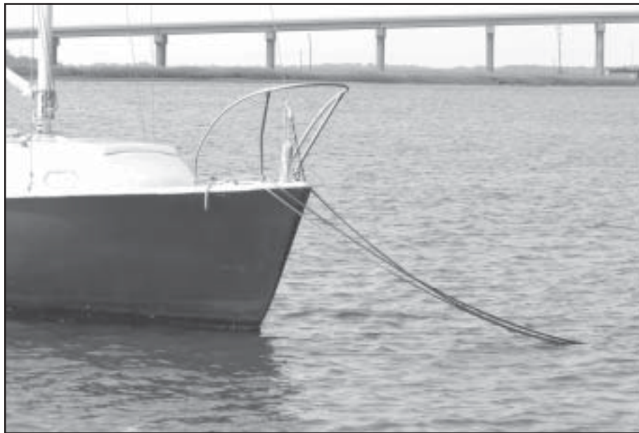
Simple redundancy—as displayed above—is one way to enhance holding power, but it's rarely the most efficient approach to anchoring.
