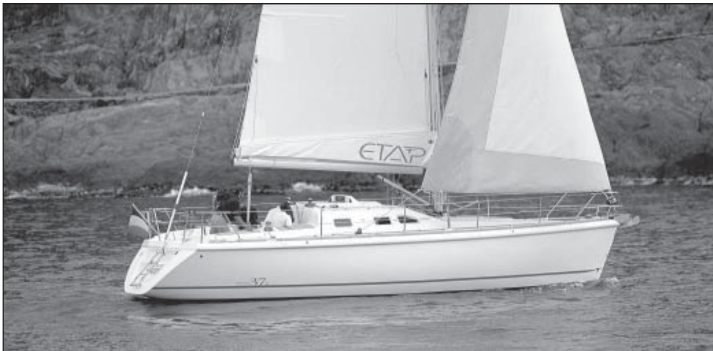
The pilothouse integrates nicely into the deck design on the Etap 37s, but the lifelines seem too low.
