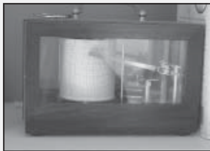
The traditional barograph (left) is a valuable tool for navigation, but it can fluctuate wildly in rough seas. An electronic barograph (right) isn't affected by the boat's motion. The one aboard Starr Trail was pivotal in the boat's success.
