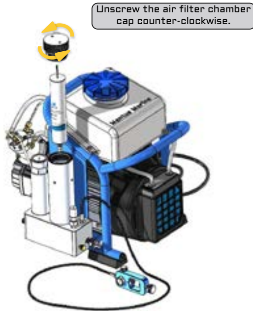
Fig 12. Changing the Triplex Air Filter
